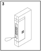
Using a bradawl mark all centres (+) on template. Remove template from door.
