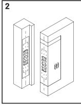
Mark height on door and frame then secure template with tape.
