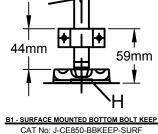
CAT No: J-CE850-BBKEEP-SURF ALTERNATIVE SURFACE MOUNTED BOTTOM KEEP (SUPPLIED WITH METAL DOOR VERSION)
